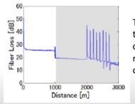
The OTDR offers the measurement of trunk and reflection peaks of branch paths.
